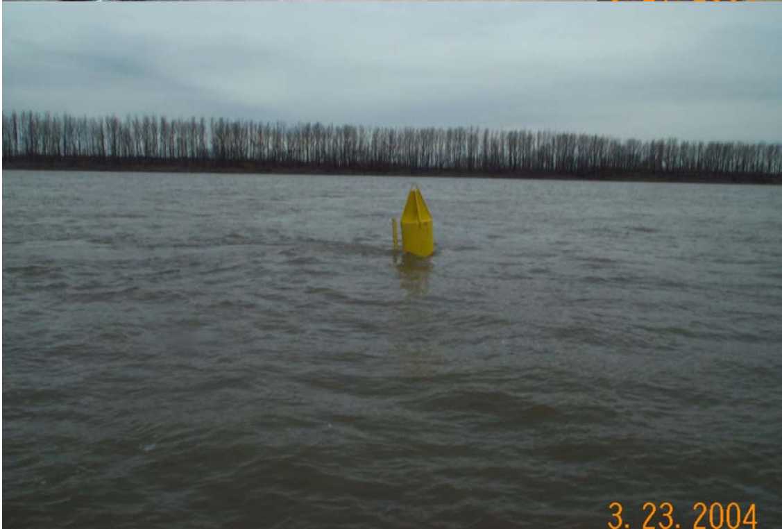
Appendix A-33. Navigation buoys modified, painted, and deployed to house VR2 (Vemco, LTD.) stationary receivers in the middle Mississippi River from spring 2003 through 2005.
