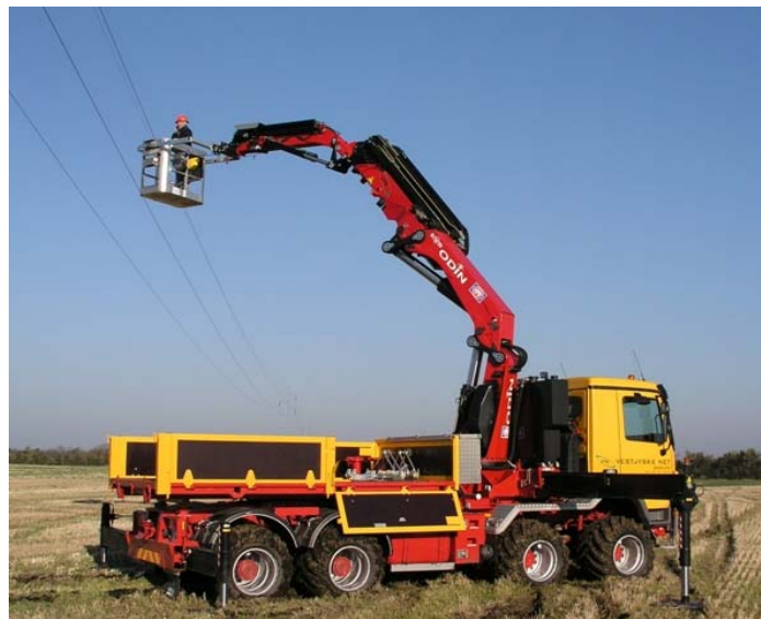
Fig. 1: Truck with loader crane used for personal lift.
