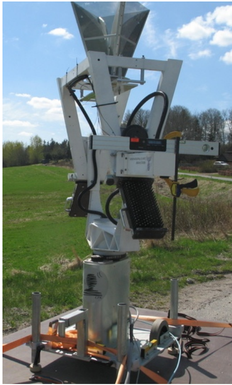
Fig. 2. The dual-polarized horn antenna mounted on the pedestal controlling the direction of the horn.
