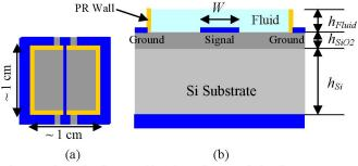
Fig. 1. Schematic of an on-chip microstrip transmission line. (a) Top view. (b) Cross-section view. Drawing not to scale.
