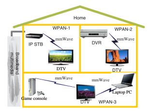
Fig. 1. Configuration of Gigabit WPANs.
