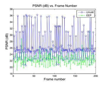
Fig. 9. PSNR as a function of the video frame number under random uniform error case.
