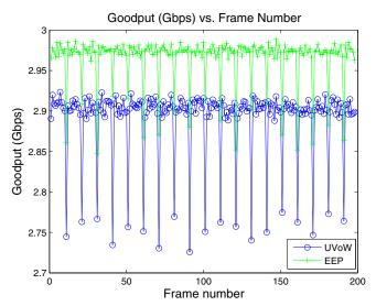
Fig. 10. Goodput as a function of the video frame number under burst loss case.
