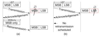
Fig. 6. UV-ARQ protocol sequence: If LSB portion is received in error then no retransmission is scheduled.
