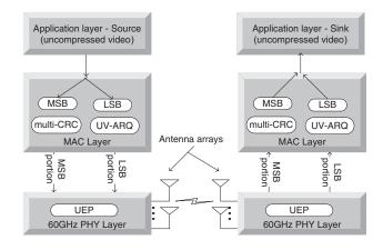
Fig. 2. UVoW system architecture.
