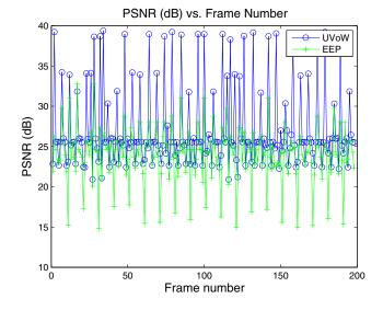
Fig. 11. PSNR as a function of the video frame number under burst loss case.
