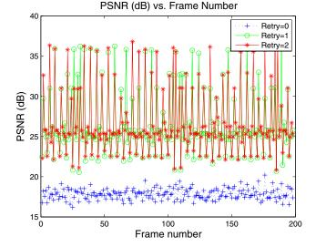
Fig. 7. The effect of the number of retransmissions on the PSNR. Results for the UVoW are shown.
