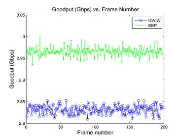
Fig. 8. Goodput as a function of the video frame number under random uniform error case.
