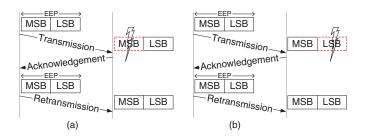
Fig. 5. Traditional ARQ schemes use single CRC. Even partial bits are received correctly; the sender retransmits another copy of the original packet.
