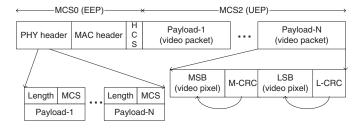
Fig. 4. The frame structure used in the UVoW.
