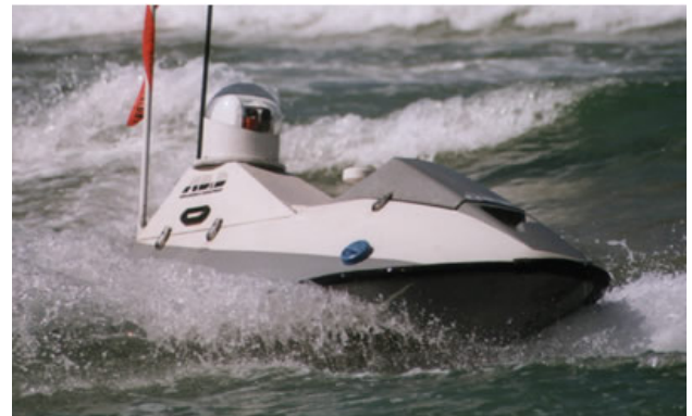
Fig. 1. The Unmanned Surface Vehicle (USV) Stingray by Israeli based Elbit Systems in action [3].
