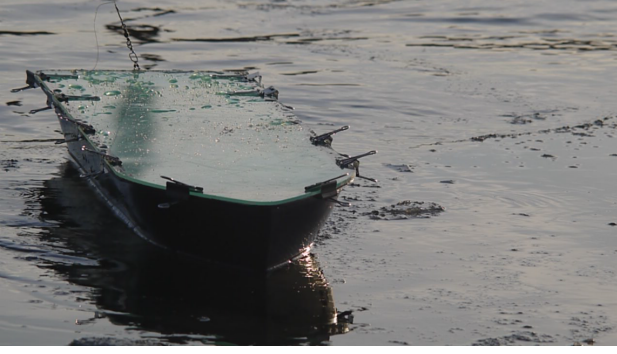
Fig. 2. AAUSHIP.01—a prototype of an autonomous maritime surface oceanographer, as this is only a prototype, the lid is held in place with clamps.
