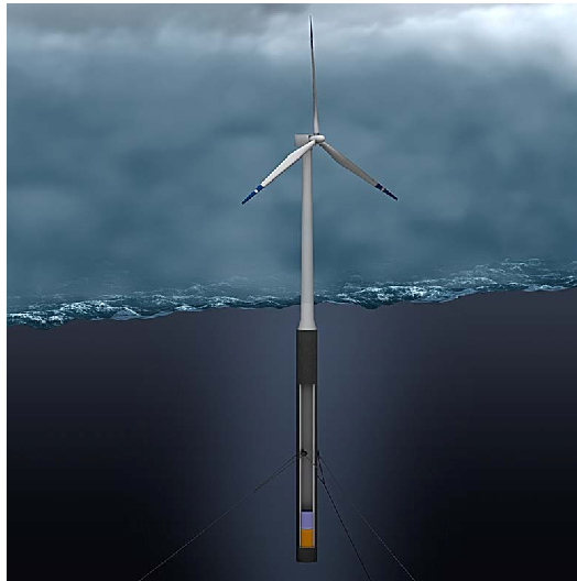
Figure 5.1: 5MW ballast-stabilized floating wind turbine. ©2011 by Statoil.
