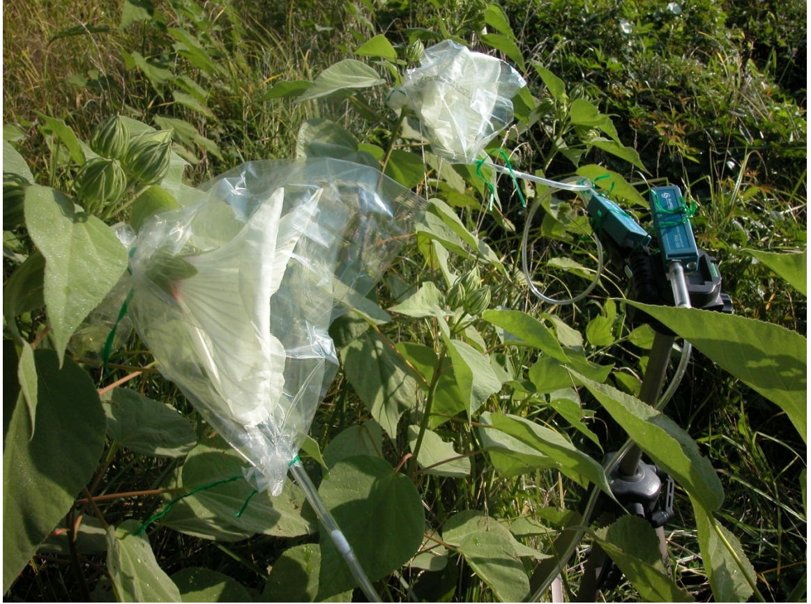
Figure 4. Floral scent collection apparatus for dynamic headspace sampling.
