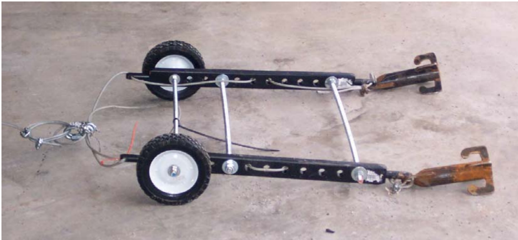
Figure 3. Rig used to grapple line between anchor and stand (see Figure 2).
