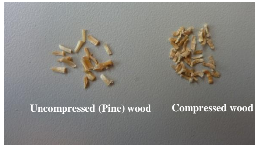
Figure 20. Compressed and uncompressed samples for TG analysis
