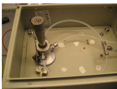
Figure 7. Quartz glass burner with two inlets
