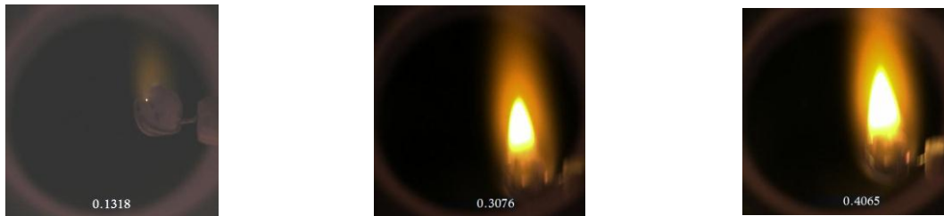
Figure 28. Ignition of a spherical particle ( d_p=3\text{mm} ) in the reactor ( T=1200^\circ\text{C} and \text{O}_2=21\% ).
