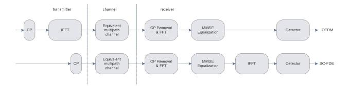
Fig. 2. System Diagrams of OFDM and SC-FDE.
