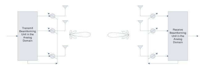
Fig. 1. Illustration of the antenna array beamforming.
