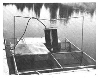
A modified Pennsylvania light trap, with the funnel removed, suspended vertically over the center of a compartmentalized cage.
