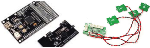
Figure 4: Left, the elements of the base-station, a CUI32Stem and a ZigFlea board. Right, the Grove I2C touch sensors with included touch sensor feelers.
