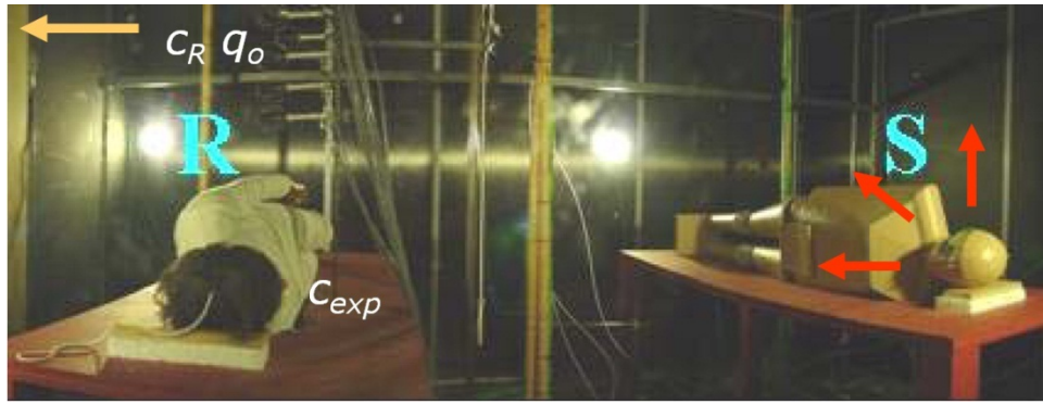
Figure 2. Two patients (life-size manikins) in a hospital ward. One patient is the source of airborne infection (S), and the other patient is the recipient (R).
