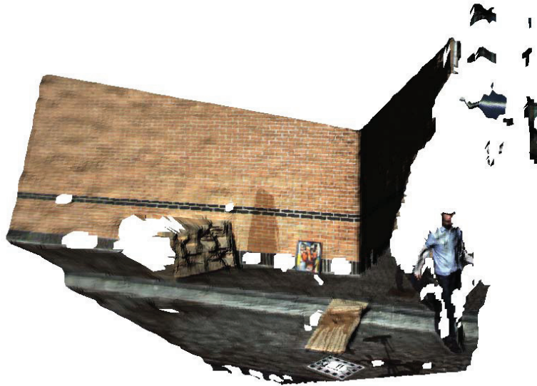
Fig. 2. Textured 3D scene mesh generated from stereo disparity information from the image shown in Figure 1. Notice how well the main surfaces in the scene are reconstructed
