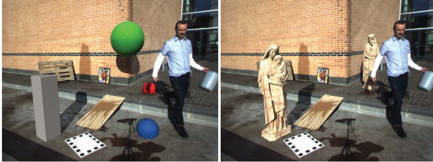
Fig. 1. Two different augmentations into frame 139 of a 200 frame sequence. The statue, the diffuse grey box and the three glossy spheres are rendered into the scene with illumination estimated from the shadow cast by the walking person.
