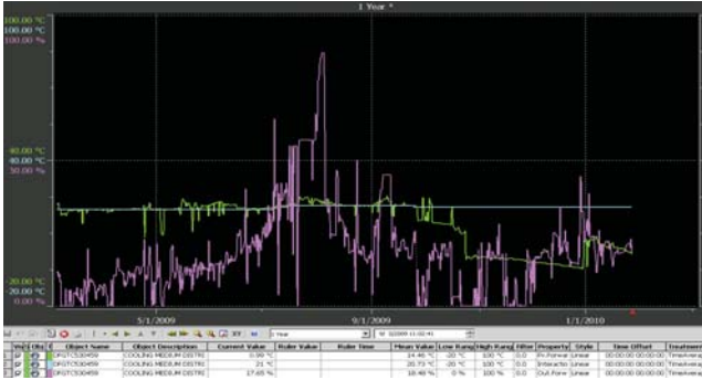
Fig. 3. Recorded seawater temperature and openness degree of TCVs
