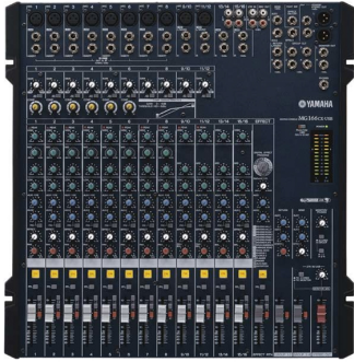
Figure 1: The traditional mixing console control surface consists of sliders, knobs and buttons. Each vertical bar represents an audio channel with controls for volume, panning, filtering/limiting and aux sends. (Pictured is the Yamaha MG 166CX USB).
