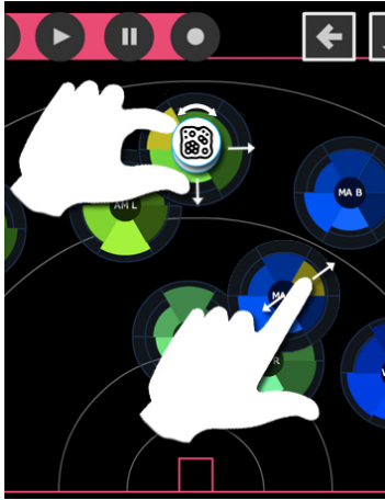
Figure 4: The initial mixing interface lets users control audio channels by manipulating widgets on an interactive surface using the stage metaphor. The position of each widget relative to the listening point determines the volume and panning of the associated channel. Widgets can be controlled using multi-touch, TUIs on all widgets, Few TUIs that are only deployed when needed, or using a smart tangible. See the interface in use at http://youtu.be/9WAI3FCzugE
