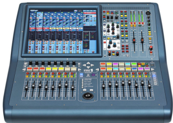
Figure 2: The digital mixer still implements the channel strip control structure where each audio channel is organized as fixed columns with sliders, knobs and buttons as main control devices. (Pictured is the Midas Pro1 IP).
