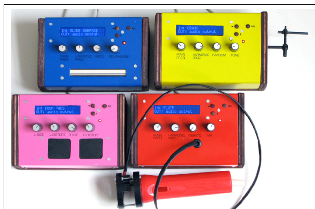
Figure 1. The PHOXES system is modular and currently implements four different modules each implementing a different physical model and a different excitation controller. Upper from left: friction PHOX and particle PHOX. Lower from left: drum PHOX and tube PHOX.
