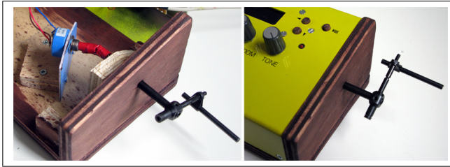
Figure 3. The crank is used as excitation controller for the particle PHOX. It is attached to a multi-turn rotational potentiometer.
