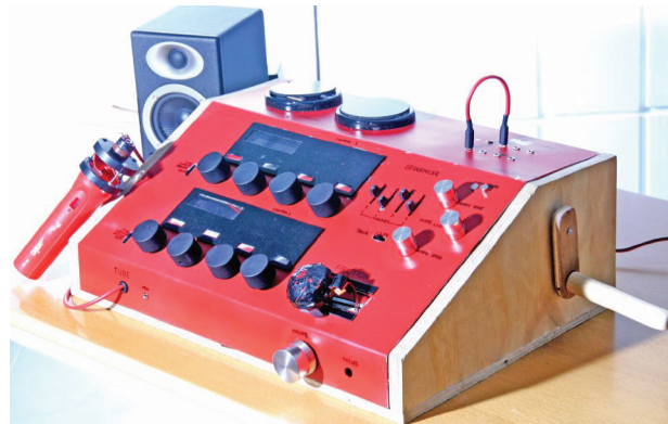
Figure 2.1: The PHYSMISM is a digital instrument for creative exploration of physical models.
