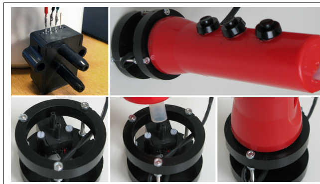
Figure 2. The flute controller is implemented using an amplified low pressure sensor mounted to the end of a tube, which the user blows into.
