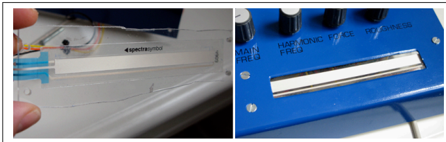
Figure 4. The friction PHOX implements a ribbon sensor, which lets the user slide his or finger back and forth over the surface to create energy.
