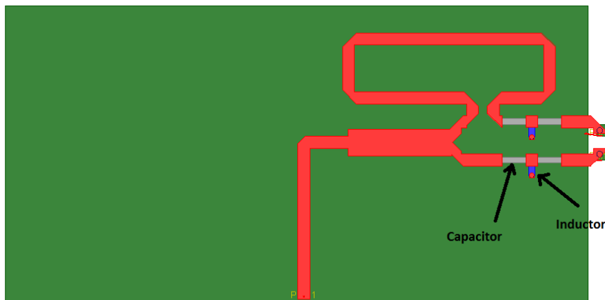
Fig. 4. The layout model of the feeding network used in the method of moments simulation. Red represents top layer whereas green represents the bottom layer with FR4 in between.
