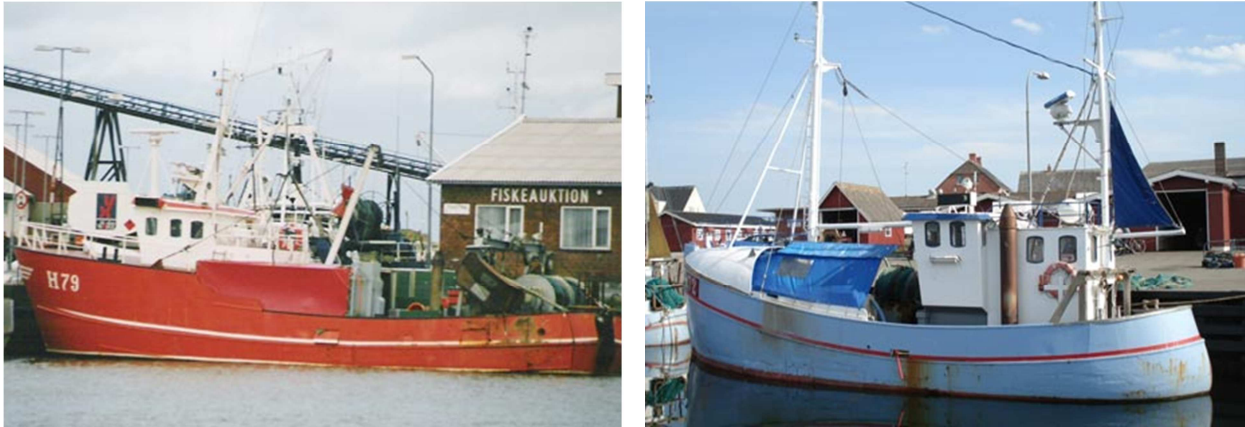
Figure 1: 2 Kattegat nephrops trawlers; H79 Tiki (steel 17 m) and FN272 Tina Malene (wood 14 m),
