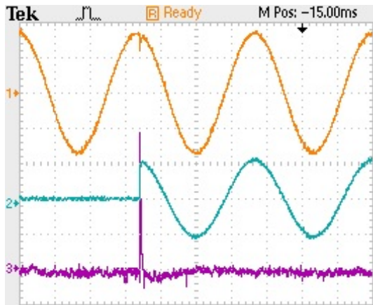
Fig. 20. Transient waveforms in response to no load to nominal resistive load step change: Ch1 denotes the output voltage (100 V/div), Ch2 denotes the load current (20 A/div), and Ch3 denotes the tracking error (10 V/div).
