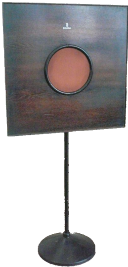
figure 4: Siemens speaker 1937, 5 Watt
