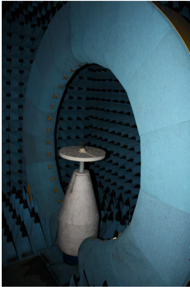
Figure 2.1: The measurement platform placed in the anechoic chamber on Satimo positioner. The cross-shaped probes are also visible in the SG32 measurement arch.
