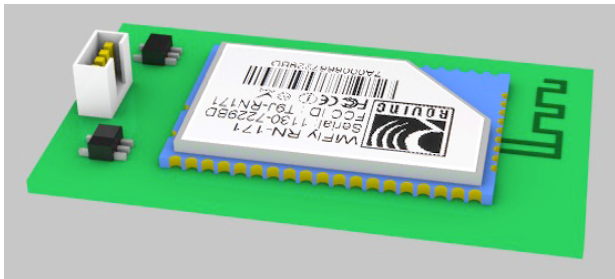
Figure 4. Rendering of the WiFly 802.11b/g radio module developed by Tobias Thyrrestrup - this will be available from Seed Studio as the ‘Serial WiFi’ GROVE element
