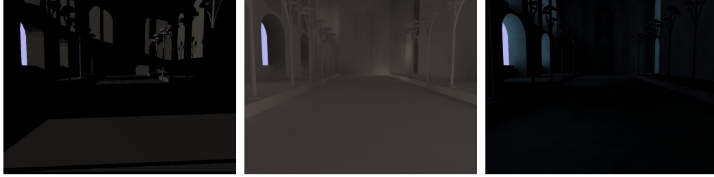
Figure 3: The different elements that make up the final result. Left: direct illumination (computed at runtime). Center: indirect illumination (precomputed at several time steps). Right: skylight (precomputed once and scaled)
