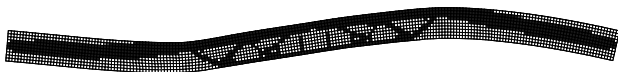
Fig. 4 Asymmetric bifurcation buckling mode of optimal design from optimization 4 on symmetric model.
