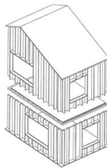
Prefabricated box elements are lifted into place and assembled on site. (KLH 2011)
