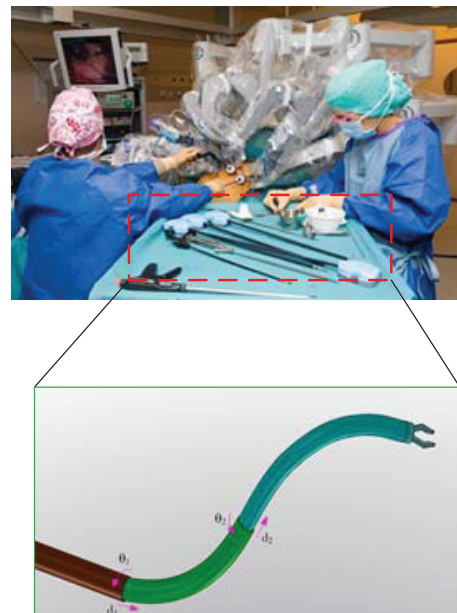
Fig. 1. A da Vinci training robot with straight-shape instruments, comparing with a continuum robot
