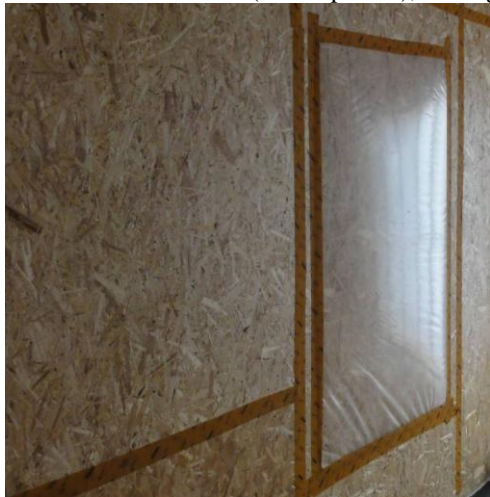
Fig. 8. Airtightness of an open OSB boards, measured by blower door test. A PE-foil is placed on the board to illustrate the openness of the boards.
