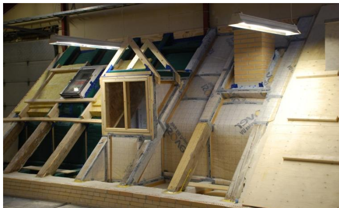
Fig. 7. Mock-up to resemble refurbished attics. Blower door tests were performed to test the airtightness of different vapour barriers.
