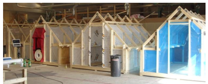
Fig. 6. Small test buildings where the airtightness of the vapour barrier was tested by the blower door method with a pressure difference of 50 Pa.
