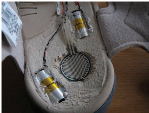
Fig. 2. A picture of one pressure sensor and two actuators embedded in the shoe in correspondence to the heel.
