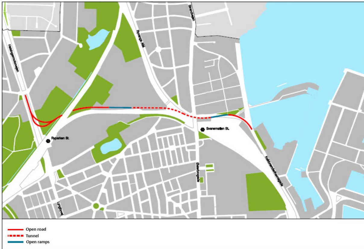
Figure 41: Alignment used for the Nordhavnsvej case (Tetraplan 2011). The proposed project offers a direct link between a busy motorway in the north-west and a new residential area planned at the harbour area to the south-east.
