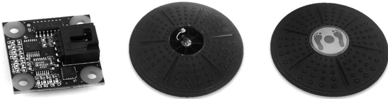
Figure 4. Left: The Phidgets accelerometer used to measure the tilt angle of the wobble board. Middle: The accelerometer attached at the center of the board. Right: Since the placement of the accelerometer dictates the heading of the tilt, it was necessary to add an icon that indicated how users should position themselves on the board.
