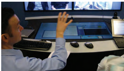
Figure 5. Table rim in BISi designed to accommodate keyboards, pointing devices as well as laptops that people might bring into the collaboration without interfering with the touch surface.
