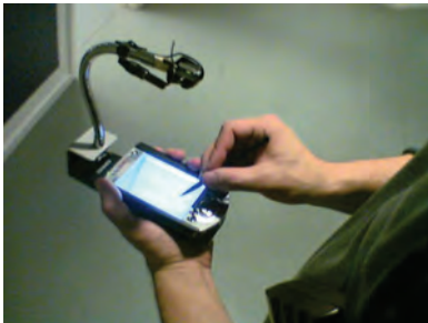
Figure 14. Wireless camera mounted on PDA
