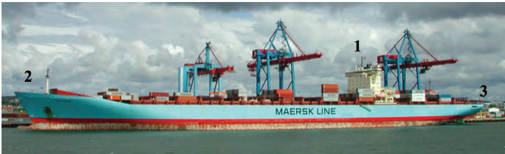
Figure 2. Sine Maersk (347 m. long and 43 m. wide) in Gothenburg Container Terminal, Sweden
