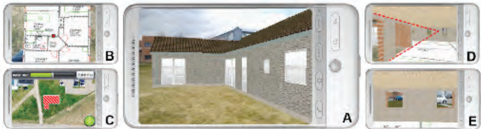
Figure 2. ArchiLens - A: Screen capture of a virtual house positioned on a lawn. B) Screen capture of the Blueprint View, showing a general overview of the floor plan. The red square represents the user's position on the blueprint. C) Placement View for house placement and rotation. The red shape represents the house, and touching the screen makes it possible to rotate the house. D) View from inside the house. Notice the added dashed dividing lines between the roof and walls moving inwards and thereby creating perspective. E: Future view through the windows of the living room. Notice how the physical surroundings are visible through the windows in the virtual walls.
