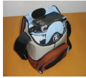
Figure 11. Our most recent version of the field laboratory weighing only 2 kg and measuring just 18x14x25 cm - containing video and audio receivers, Picture-in-Picture unit, hard disk recorder, and battery.
