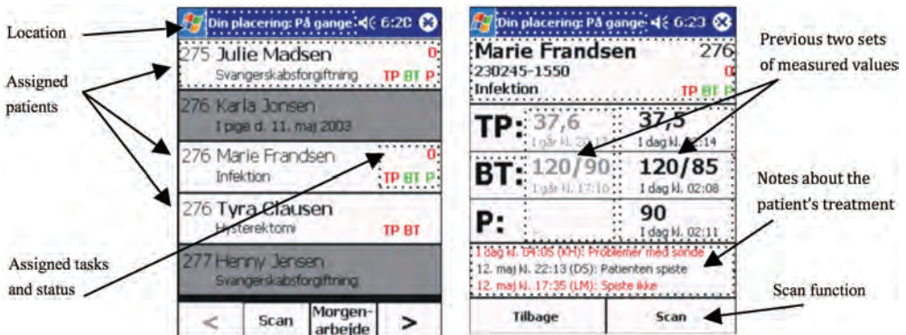
Figure 4. Interface layout from MobileWARD illustrating patients admitted to the hospital (left) and information on a selected patient (right).
