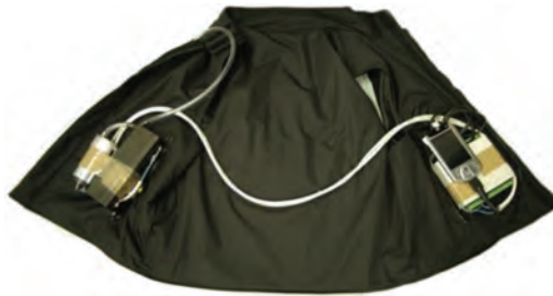
Figure 8. Hug Over a Distance prototype: showing pump, valve, battery, relay controller and wireless PDA. During use, these components are hidden inside the vest.
