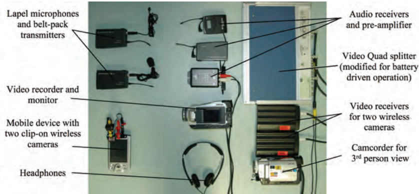
Figure 5. Equipment used for the second field laboratory (configured for two wireless cameras). Batteries and power regulators are not shown
