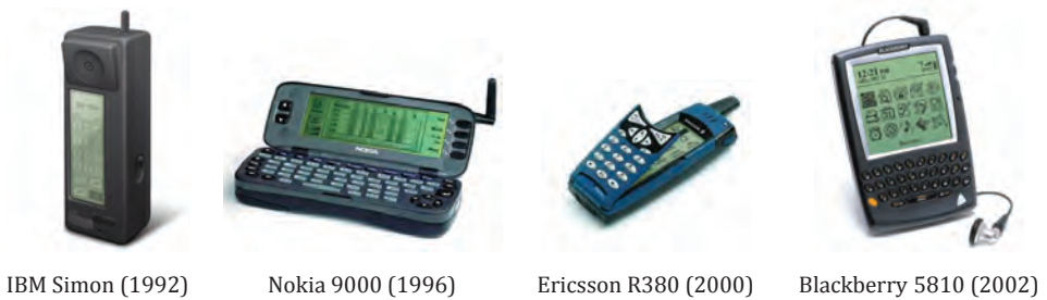
Figure 7. Smartphones exploring different physical form factors and interaction styles
