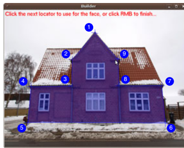
Fig. 2. Interactively defining a polygon by clicking at corresponding locators in two images. Here nine locators are used.
