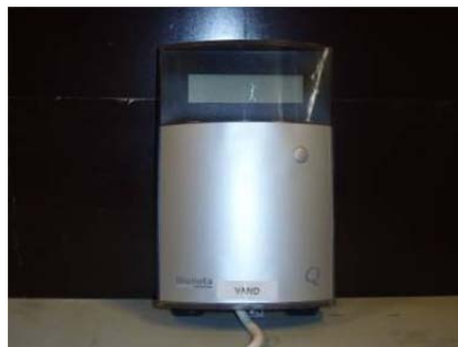
Figure B.0.4: HGQ1 heat consumption measurer.
