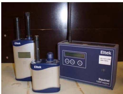
Figure B.0.3: Eltek equipment used for measuring the indoor environment.
