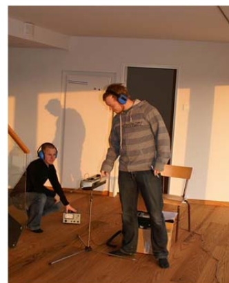
Figure D.3. Measurement of reverberation time in the Comfort Houses.
