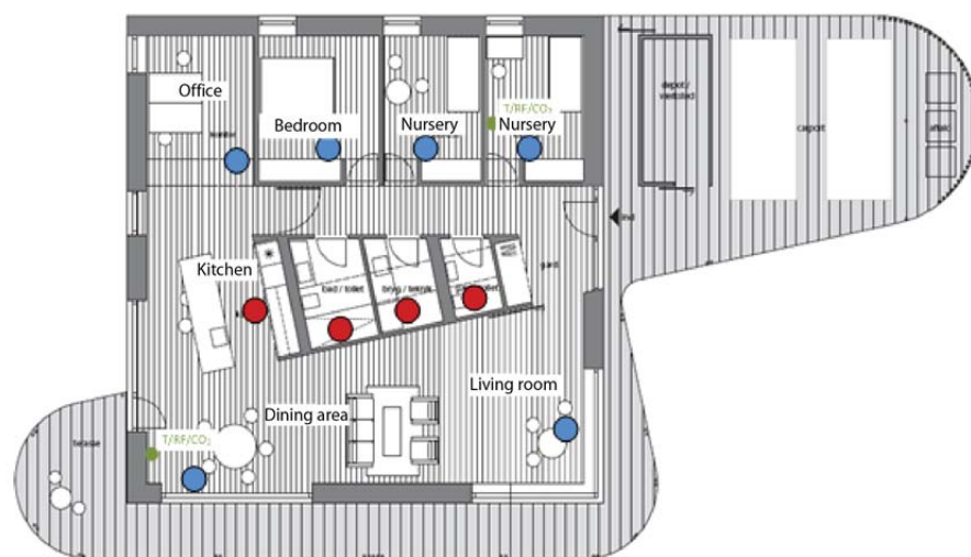
Figure 3.22. The position of the equipment measuring the temperature in living room and room (green markers) as well as the ventilation inlet (blue circles) and exhaust (red circles).
