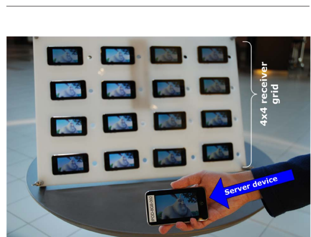
Fig. 1. Example of sharing a movie locally among mobile devices using WiFi technology for the iOS platform.
