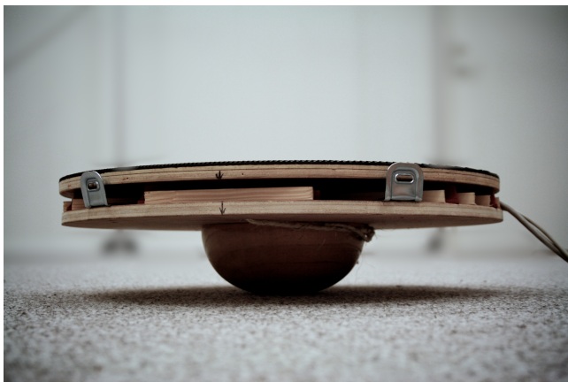
Figure 1: Actuated and instrumented wobble board.
