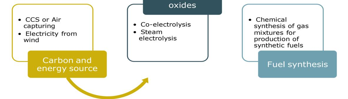
Two carbon sources are proposed - CCR from energy sector or air capturing as a promising future technology. Pathways are divided into three steps. Energy source drives dissociation of oxides, either  $H_2O$  or both  $H_2O$  and  $CO_2$ , which results in gas mixtures that are in the last step catalyzed to fuels.
