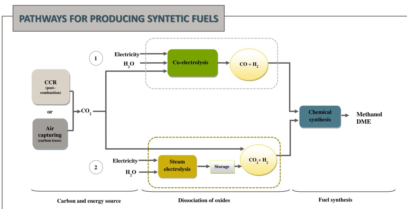
Both pathways for producing synthetic fuels exclude direct biomass input for fuel production. However, these pathways are in strong connection with power and heat sector that uses biomass
