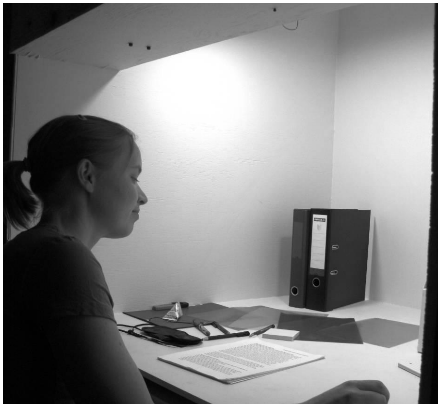
Figure 7: Subject performing the adjustment task for preferred CCT while reading a text in the scale model.
