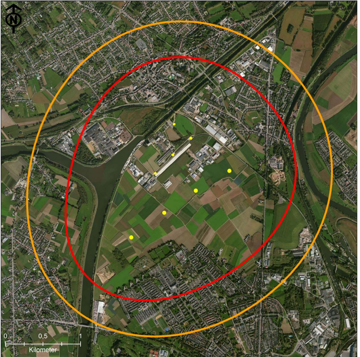
Figure 4. Contours where the 20-dB indoor low-frequency limit is exceeded in the 33% or 10-20% poorest-sound-insulated houses (red and orange lines, respectively). Wind speed 8 m/s. See text for calculation details.
