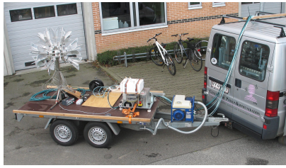
Fig. 2. Practical setup of the spherical array of dual-polarized horn antennas (in the back of the car trailer) and the four pairs of dipole antennas used for both the LTE dongle and the channel sounder (mounted on the white styrofoam).
