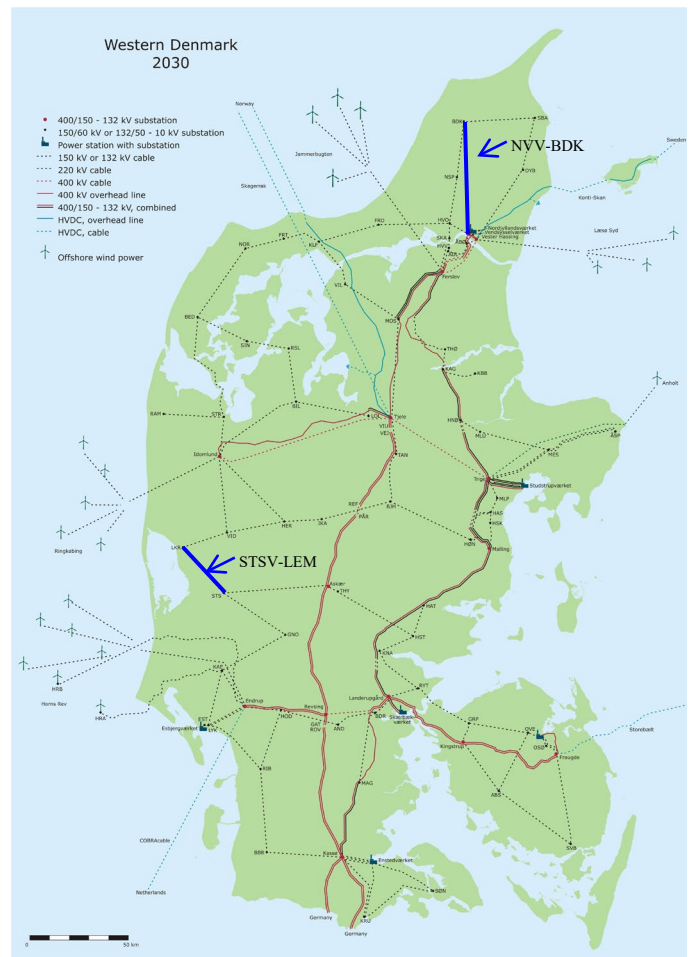
Fig. 16. West Denmark Transmission Network. Note: Due to differences between the English and Danish names of some cities, the STSV-LEM link is named STS-LKR in the map
