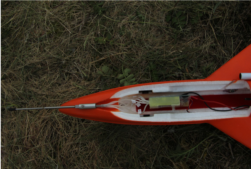
Figure 18: The 5-hole probe and its data logging system as mounted on the SUMO airframe (photo: J. Reuder).
