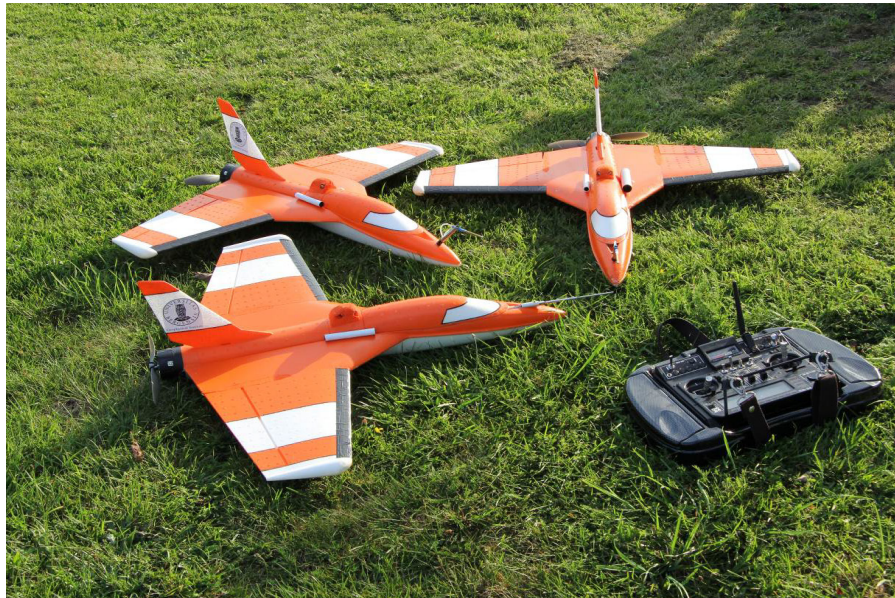
Figure 17: The 3 SUMO airframes used during the flight week. The system in the foreground is equipped with the 5-hole probe, the two in the background with the simple Pitot tubes (photo: J. Reuder).
