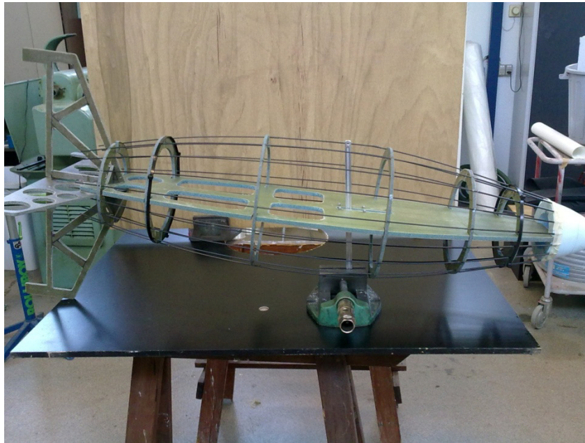
Figure 30: Zeppelin shaped canopy of the measurement platform.
