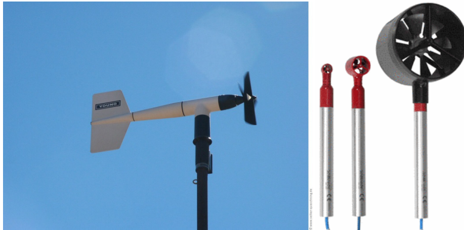
Figure 7: Two examples for propeller anemometers. Left: Young Wind Monitor 05103RM; Right: Miniaturized propeller anemometer series Mini Air from Schiltknecht.
