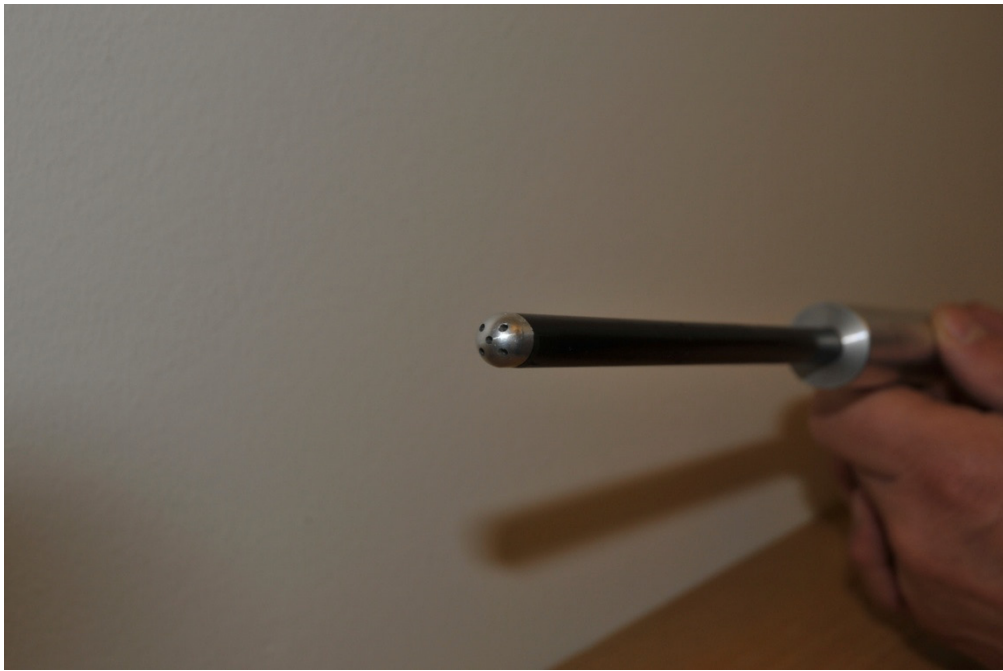
Figure 35: Five-hole pitot tube with spherical head.
