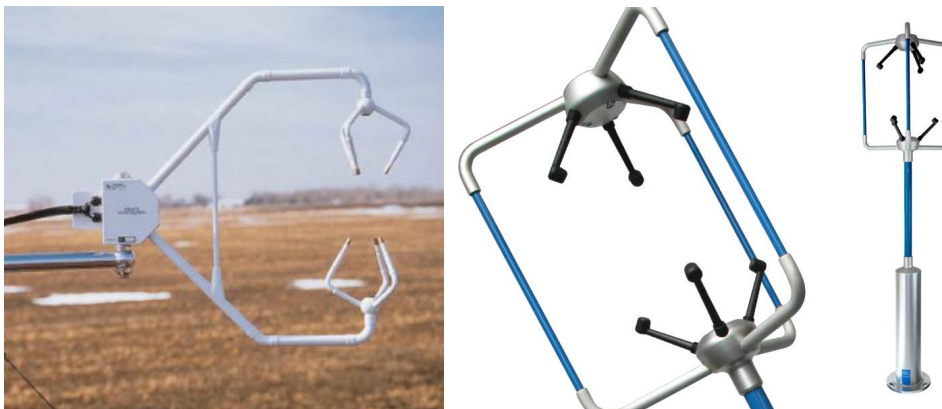
Figure 8: Two examples of sonic anemometers typically used in atmospheric boundary layer research. CSAT3 from Campbell (left) and R100 from Gill (right).
