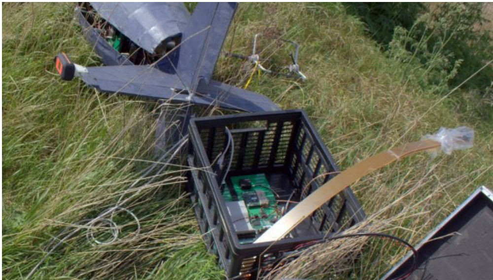
Figure 41: Picture of the base station, with GPS antenna being on an outrigger. Source: nanosync.wordpress.com
