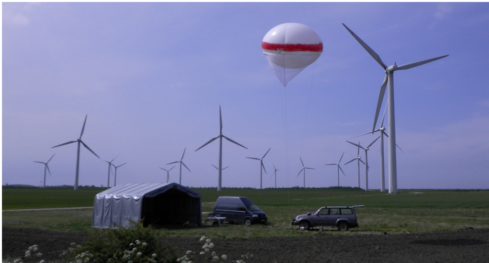
Figure 49: The SkyDoc and hangar. The winch is bolted to a steel frame fitting under the front wheel of the LandCruiser. In the background turbines of the Nøjsomheds Odde wind farm.
