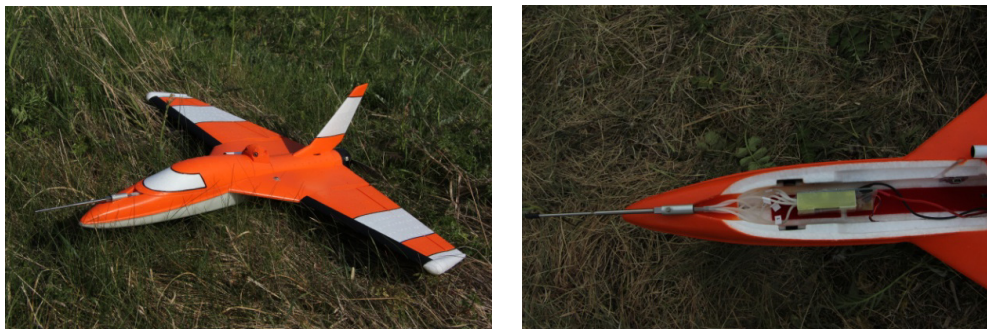
Figure 12: The 5-hole probe from Aeroprobe mounted on the SUMO aircraft. The right picture shows a detailed view of probe, tubing and the air-data computer unit inside the fuselage.
