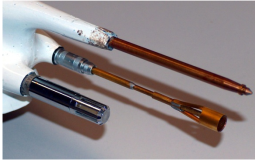
Figure 21: The meteorological package of the M2AV: 5-hole probe, thermocouple and Humicap sensor.
