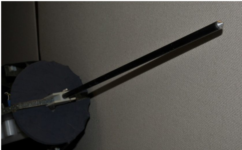
Figure 33: Close up on 5-hole pitot tube with conical head.
