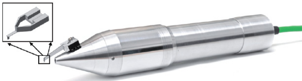
Figure 14: The 2-d Laser Cantilever Anemometer for atmospheric use (2d-ALCA) developed at the University of Oldenburg (taken from Puczyłowski et al., 2011).
