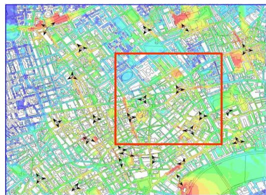
Figure 1: London Area Scenario with existing 3G site deployment. The investigated area delimited by the rectangle.
