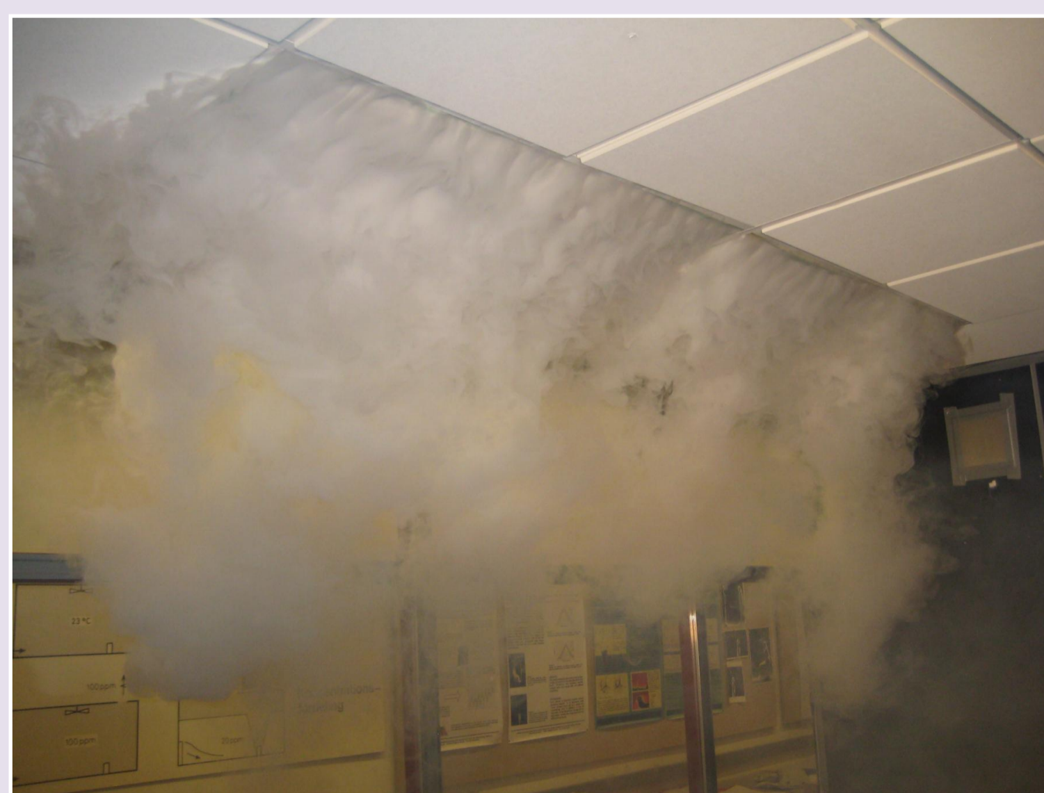
Diffuser 3. (a) Smoke visualization of the downward airflow pattern. (b) Velocity profile of the textile diffuser at three different lines.
