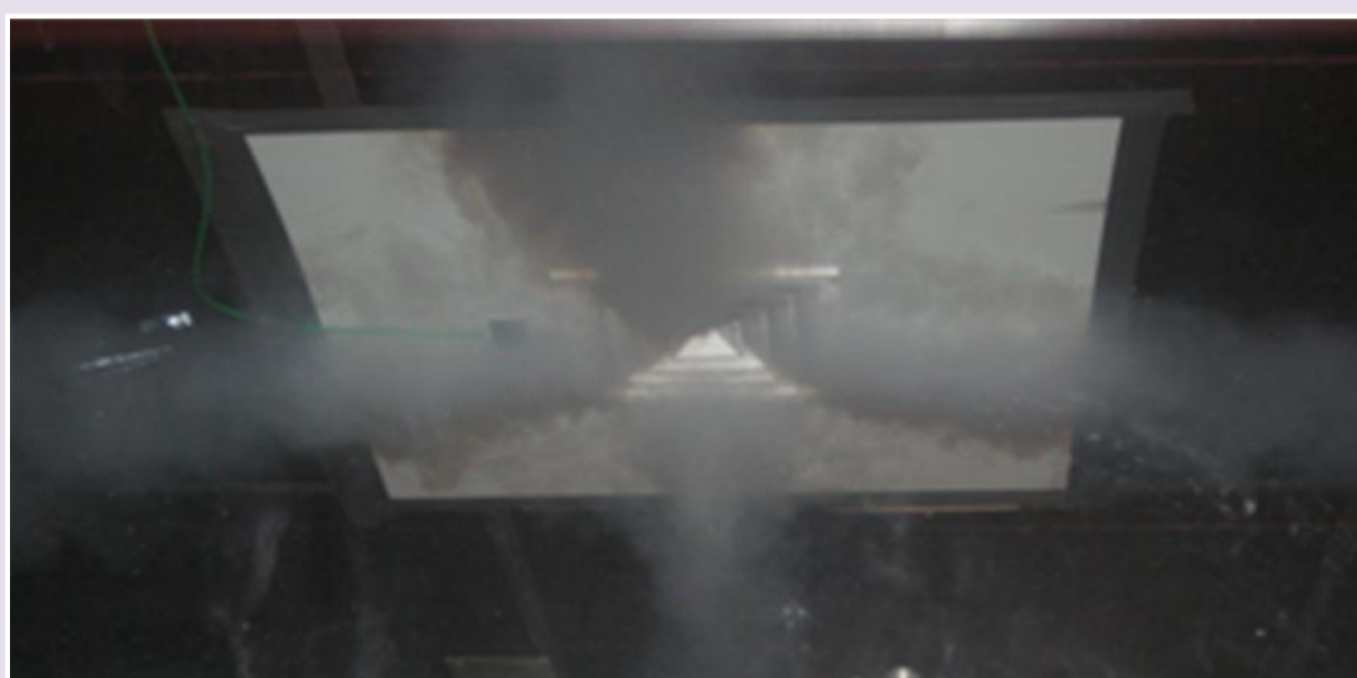
Diffuser 2. (a) Smoke visualization which shows a symmetry in the airflow generated by the diffuser. (b) Velocity measurements at lines L1, L2, L3, L4 and L5.
