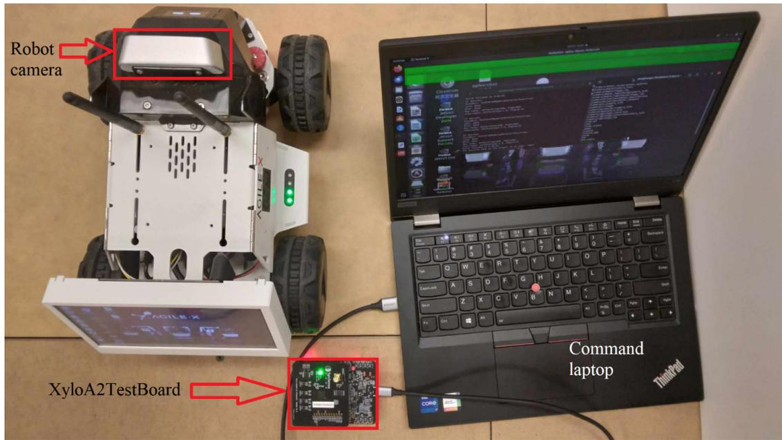
Figure 3:5: Experimental setup of a mobile robot and a Xylo neuromorphic chip.
