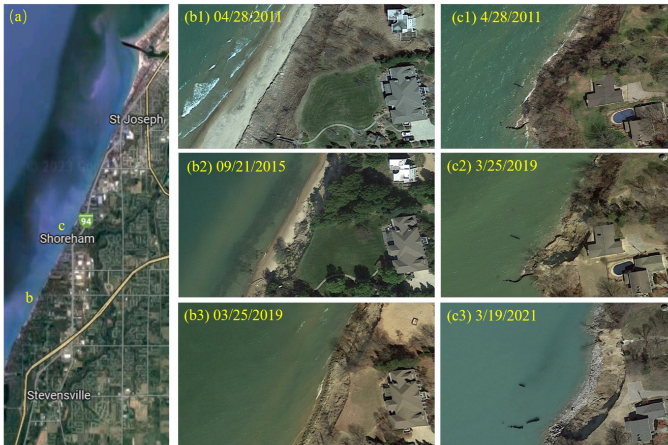
Figure 14. Illustration of two coastal erosion hotspots in Michigan along the coast of the eastern lake. (a) Location of the hotspots (b, c). (b, c) Historical satellite images (Sources: Google Earth).
