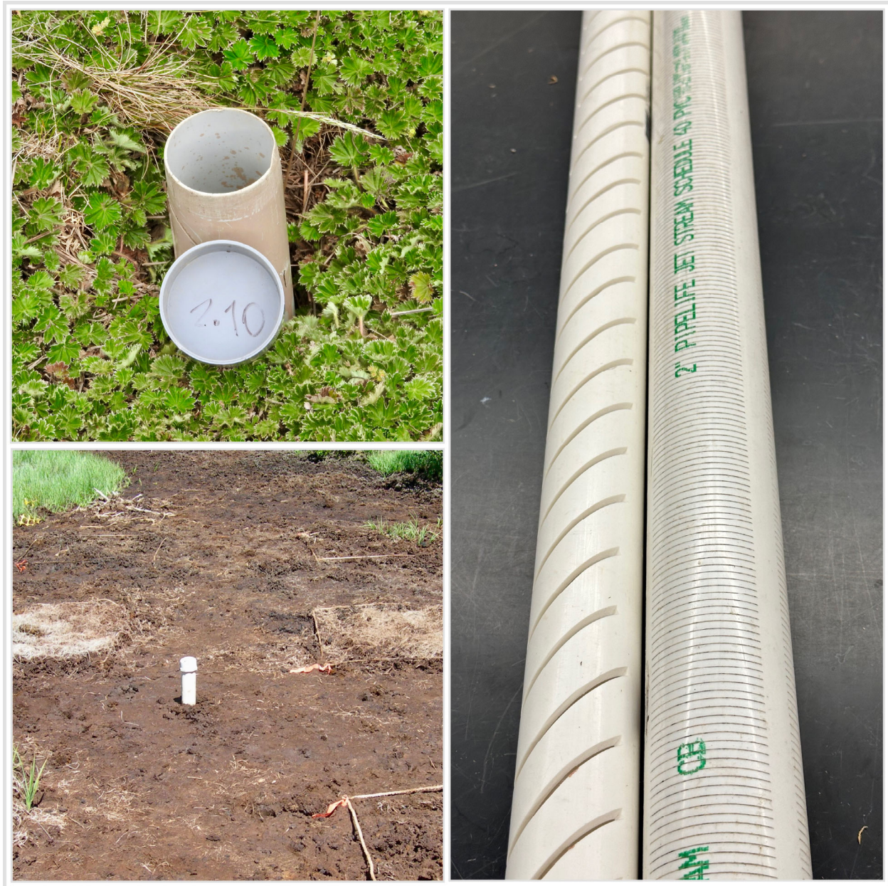
Figure 12. Groundwater monitoring wells inserted into the fen (left) and two types of slotted PVP pipe (right).
