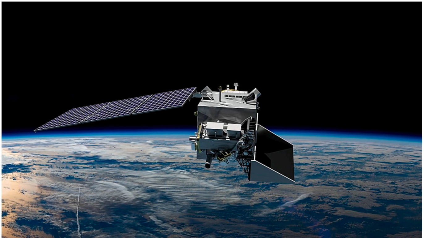
Fig. 1. Artist's rendition of NASA's Plankton, Aerosol, Cloud, ocean Ecosystem satellite flying over cloud-covered Earth's Ocean. The Ocean Color Instrument is visible on the front of the platform, while two polarimeters (located on the bottom side of the platform) are not visible from this view. Credit: NASA Scientific Visualization Studio.
