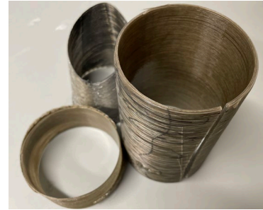
Figure 1 - 3D printed fiber-reinforced composites designed as a type of vambrace prototype for custom radiation shielding on gloved forearms.
